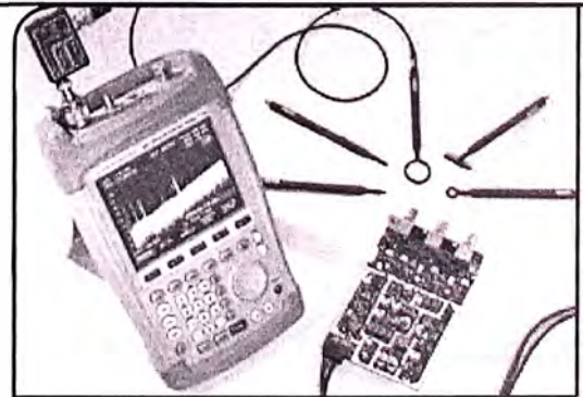
R&S®FSH with near-field probe set and DUT
