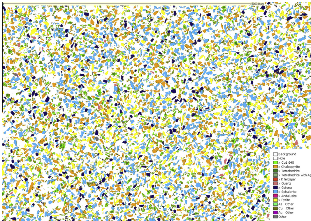
Fig. 12. QEMSCAN micrograph of leach residue.
