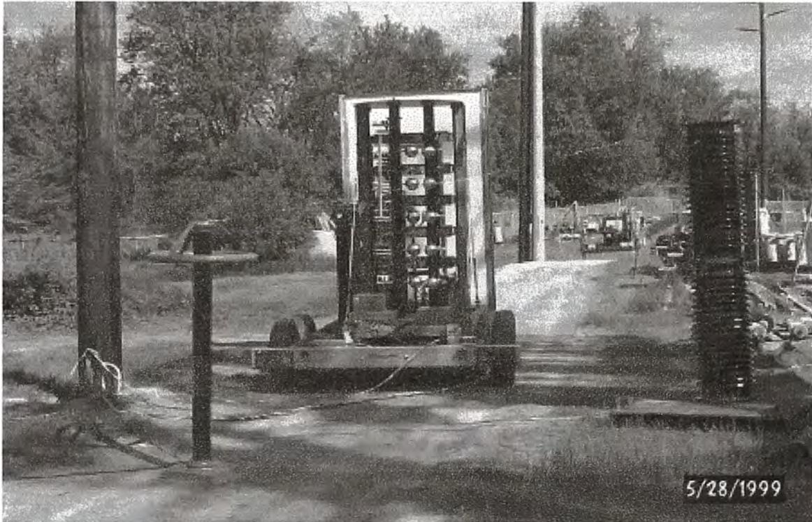
Figure 3. Photograph of the lightning impulse generator test system
