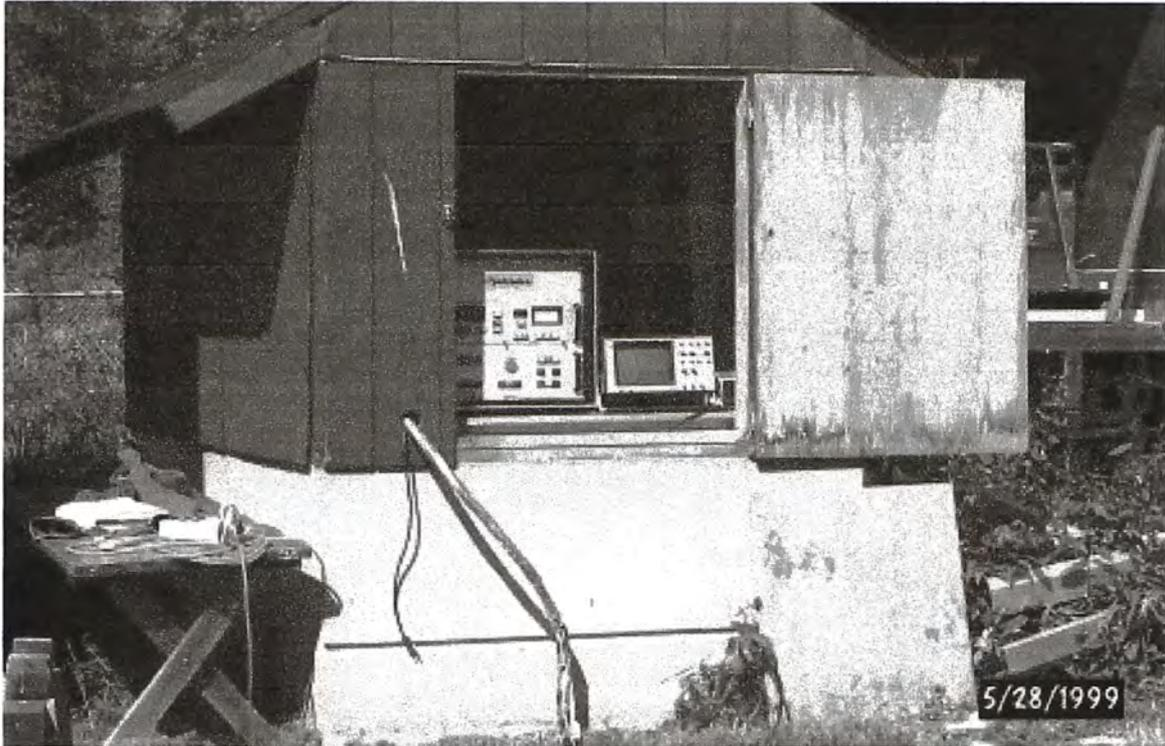
Figure 5. Photograph of the impulse generator control module and the digital oscilloscope for recording the lightning impulse wave
