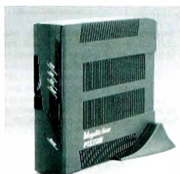
Photo 3. Customer premises equipment
