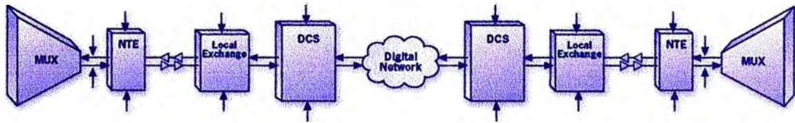
Figure 6: Possible 2.048 Mbps circuit monitoring locations
