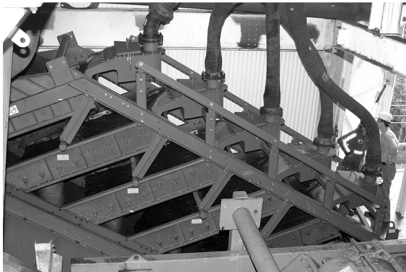
Figure 8: Stack Sizer in Operation in Eastern Kentucky, USA
