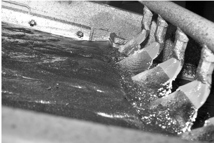
Figure 9: Polyurethane Spray Nozzles Add Approximately 40 GPM per Deck
