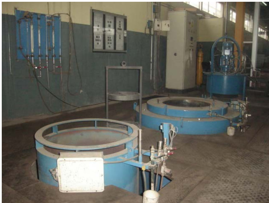
Figura 2.1. Horno de nitrocarburation.
