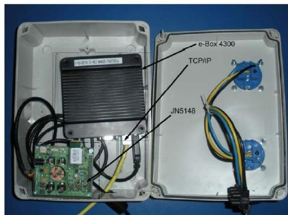
*Fuente: Street Lighting Control System Based On Large-Scale WSN: A Step Towards A Smart City (2014)*
