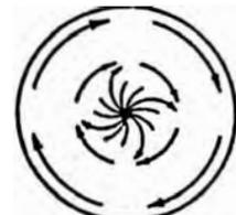
60° Lead--May give wet material maximum efficient screening pattern.
