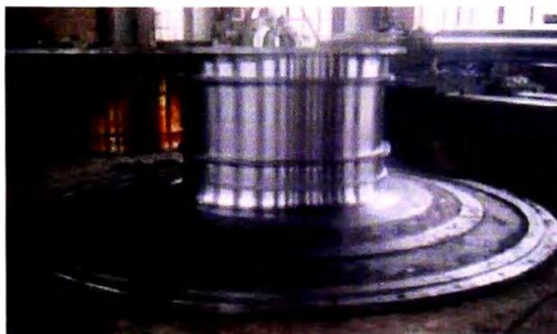
**Fig 2.13 Tapa trunnion de molino.**
