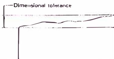
Figure B.3 — Parallelism deviation equal to the numerical value of the size tolerance
