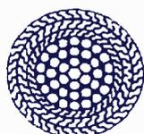
Core of helically spun round wires in several layers.
