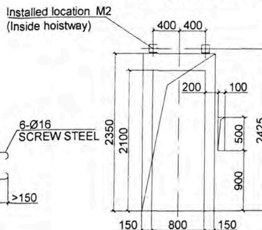
VIEW OF PRE-HOLE WHEN FIRE SERVICE REQUIRED (BASE FLOOR)
