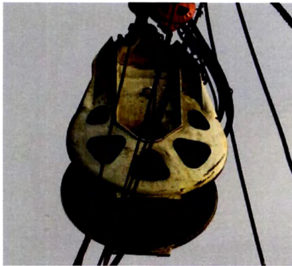
Fig. 4.7 Macaco (Power Block)
