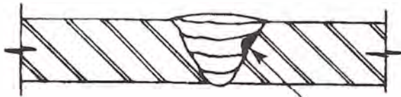
Lack of fusion between weld bead and base metal
