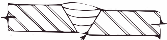
Incomplete filling at root on one side only
