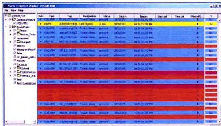
This Alarm Sequence Displays (ASD) shows all alarms in a chronological sequence. The plant topology on the left side supports fast navigations and selections. Additionally, the ASD can be displayed in Alarm Point View, which shows one line for all alarm types of an alarm source, including an alarm counter.
