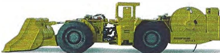
The Electrical Scooptram EST3.5 is an underground loader for small to medium-sized underground operations that include development work, production mining and construction sites. This vehicle is attractive for operations that have existing infrastructure for electric LHDs or for those that have insufficient ventilation for diesel LHDs.
