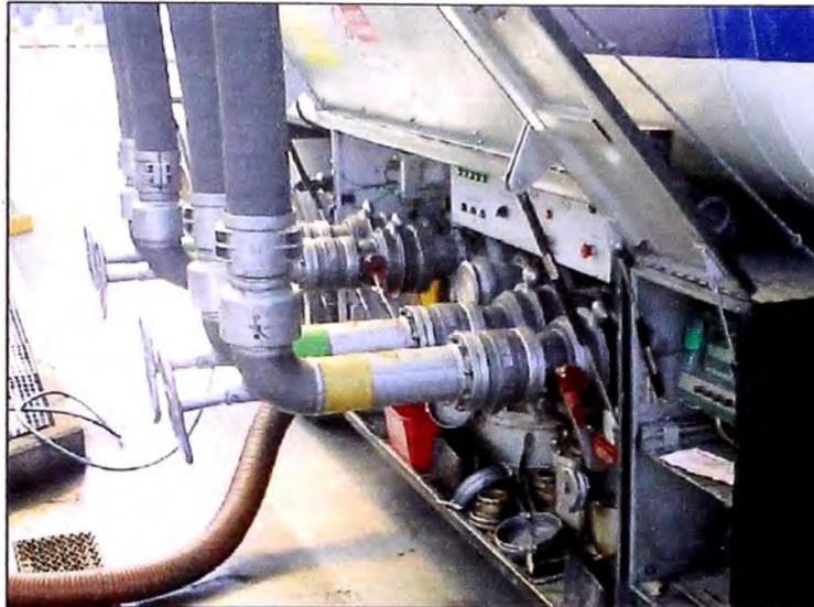
**Figura 2.5** *Sistema Bottom Loading*
