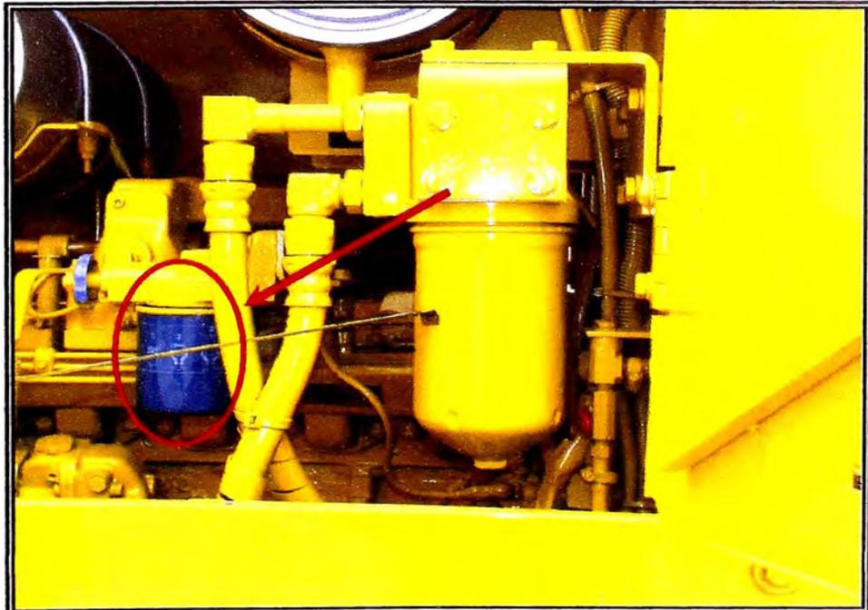
**REEMPLACE EL RESISTOR DE CORROSION CADA
