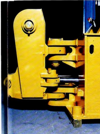
The massive fabricated swing post assembly prevents flexing when the boom is working.
