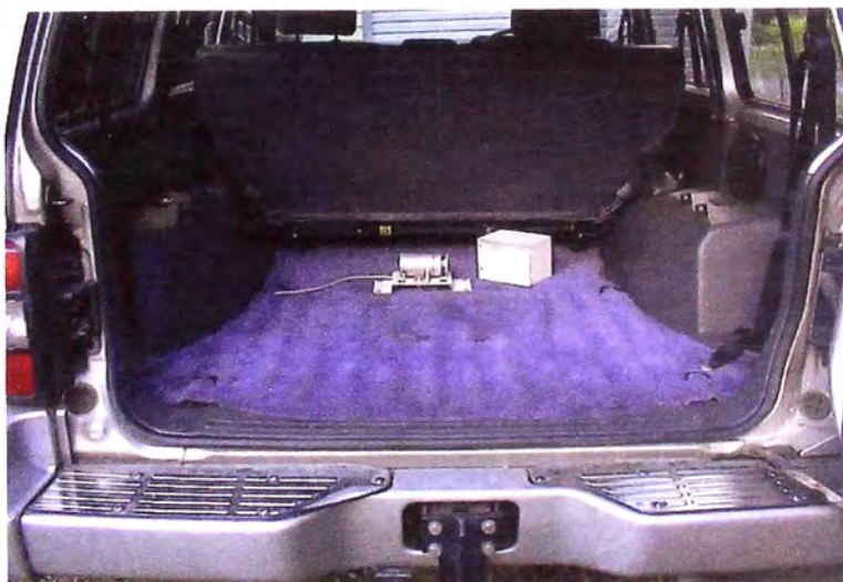
ROMDAS BI Installed in Vehicle With Protective Cover Off
