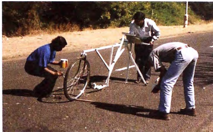
MERLIN Survey in Gujarat, India. The wood was the width of the vehicle track and the pavement was painted to precisely locate the wheelpaths
