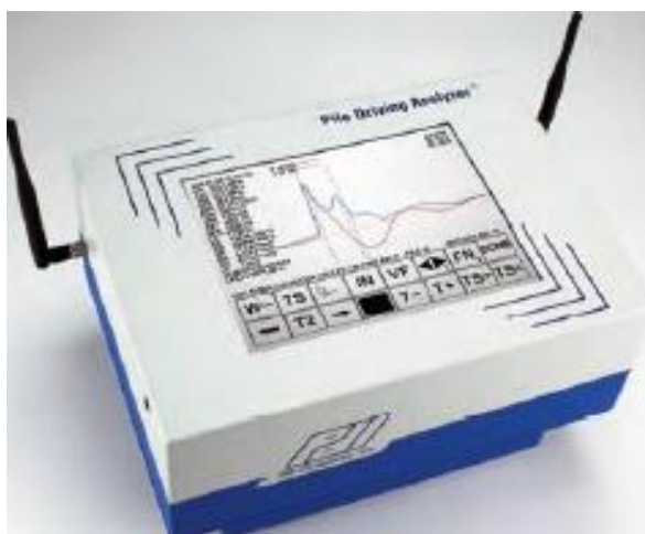
Figura N° 24 Pile driving analyzer - PDA PAX
