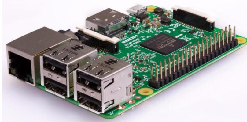
**Figura 2.5** Raspberry Pi 2 Modelo B
