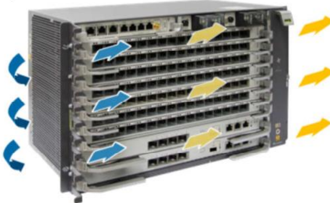
Figure 5-2 Ventilation of the MA5800-X7 service subrack
