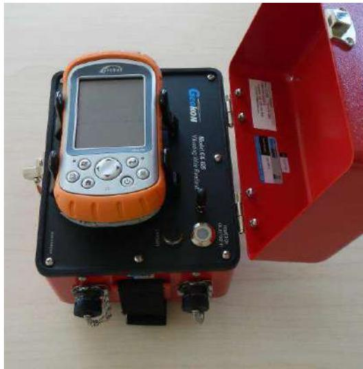
Figure 6 GK405 Readout Unit
