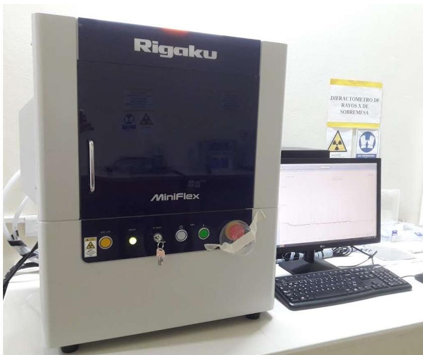
Figura 4.3: difractor de rayos X comercial Rigaku Miniflex 600.
