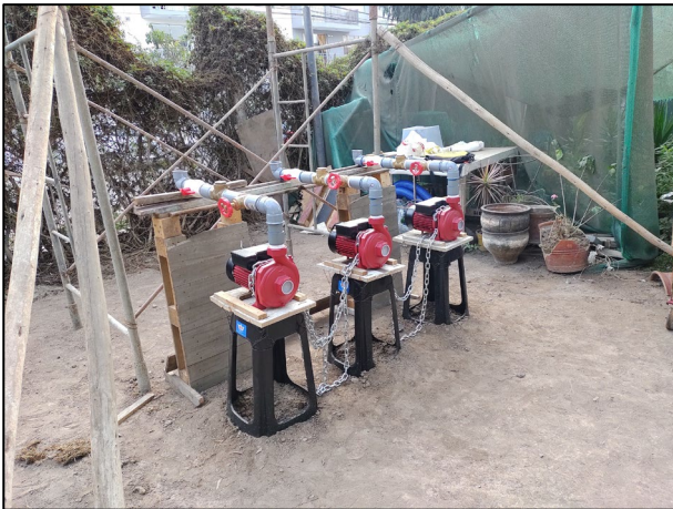
8. Bombas de 2 HP AQUAMAX \text{Ø}2 " – \text{Ø}2 "
