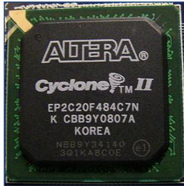
**Figura 2. 3** FPGA Cyclone II EP2C20F484C7N de Altera
