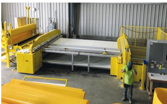
The fully automatic HDPE liner welding system from Schlüsselbauer Technology supplies liner cylinders from DN 300 to DN 1500 for a max. pipe length of 3 m.
