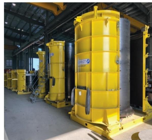
The Perfect Forming Technology moulding system for processing self-compacting concrete is a key element of the Perfect Pipe production process.
