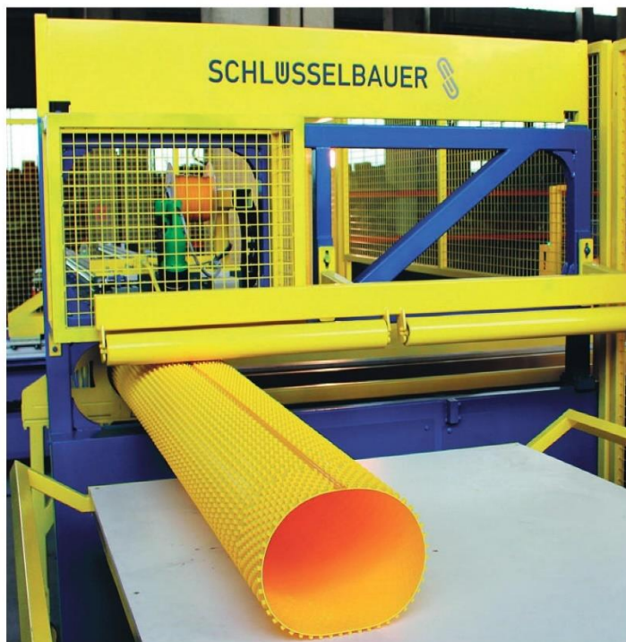
After the welding and cooling phase, the liner cylinder is ejected from the machine and is immediately ready for the next production step.
