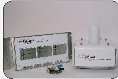
Strike Guard Sensor data are communicated via lightning-proof fiber-optic cable to an independent Lightning Data Receiver with system status, caution and alarm indicators, relays, and computer compatible output.
