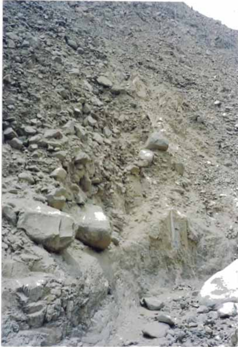
Foto 13: Quebrada Pedregal. A la izquierda se observa un depósito colgado. Apparently, the rock from the lower right corner deflected the torrent, and this, upon impact with the mass, sent the material to the slope.
