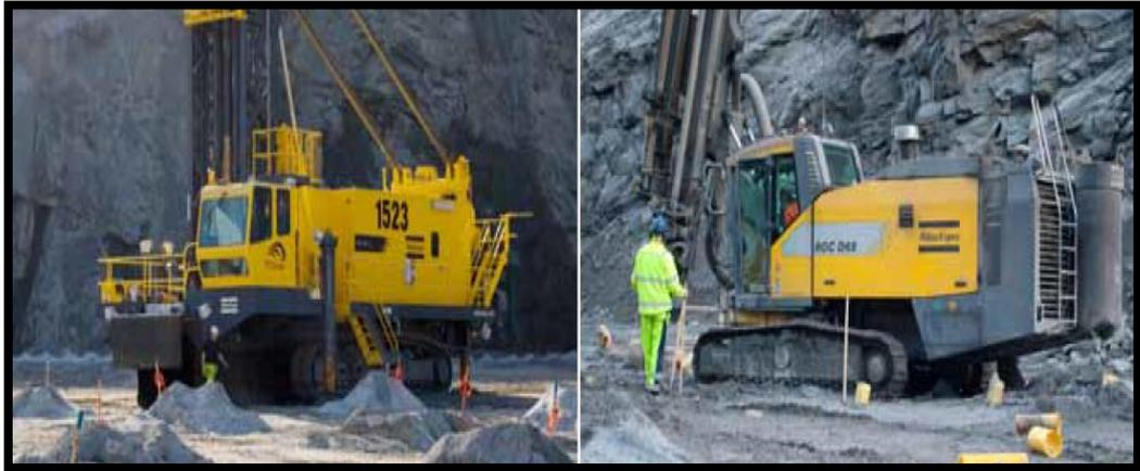
Figura 4.26 pit viper (peforadora rotativa) – (track drill) Smart rock
