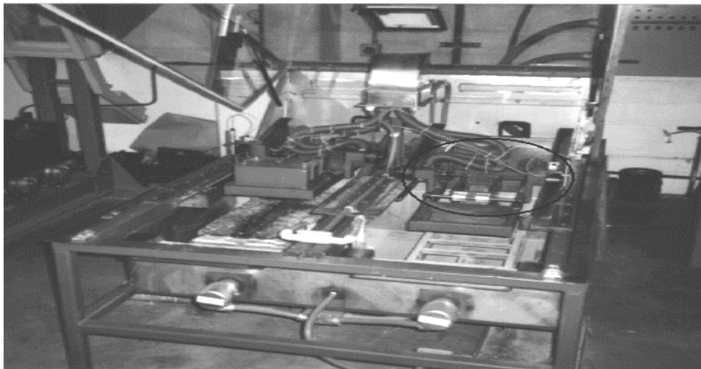
Figura 5.23: Máquina de ensayo, Purdue University Laboratory Wheel Tracking
