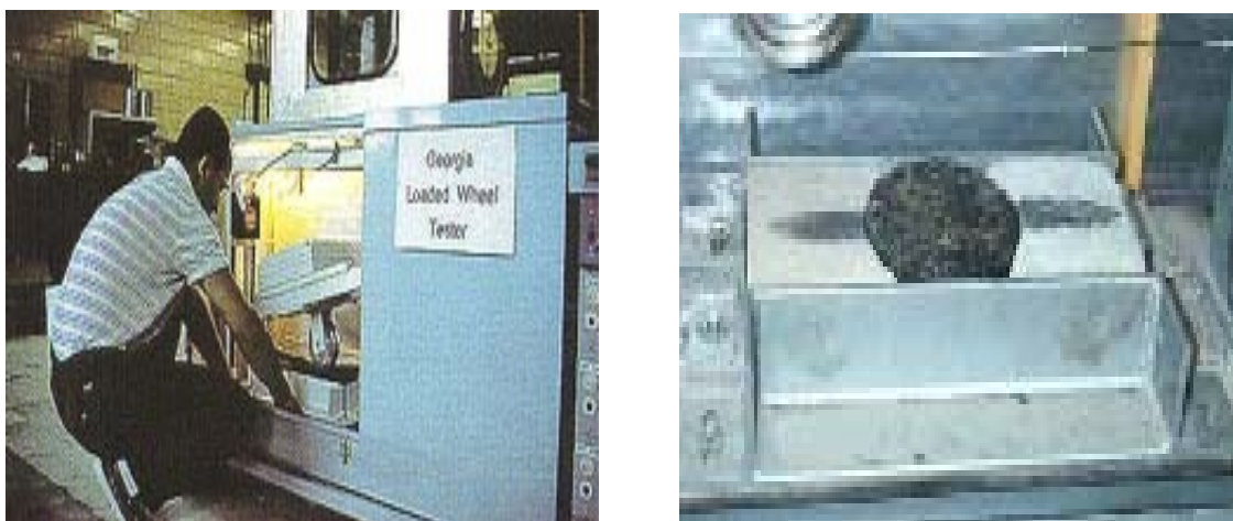
Figura 5.19: Georgia loaded wheel tester (GLWT)
