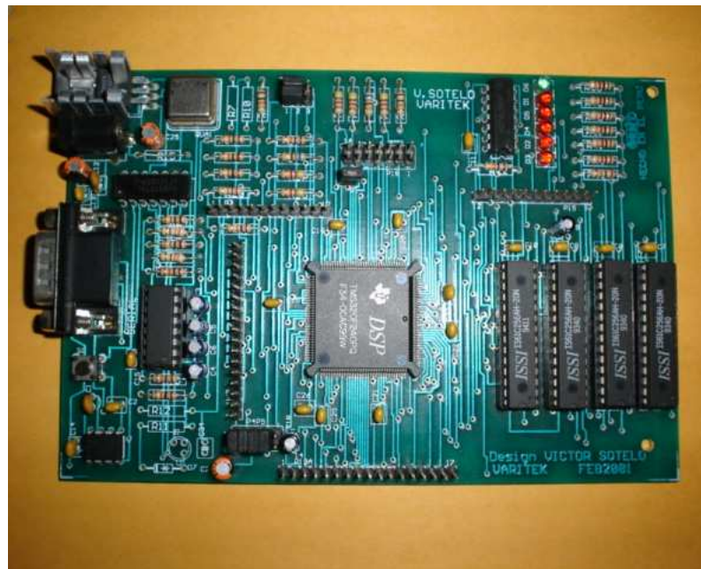
Figura 4.17: Tarjeta de control DSP - TMS320F240
