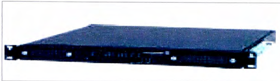
Figura 3.7 Firewall VPN Firewall Brick
