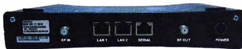
SkyEdge II IP VSAT (rear view) with Connections Labeled
