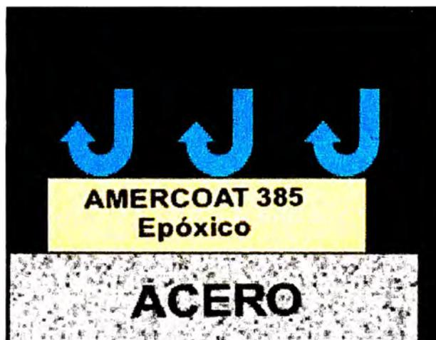
Figura 13: Pintura epoxi-poliamida amina
