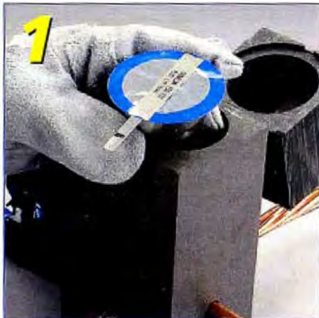
Insert CADWELD PLUS package into mold (may require use of a cover/baffle)
