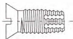
Figure 7 – Example of thread-cutting screw
