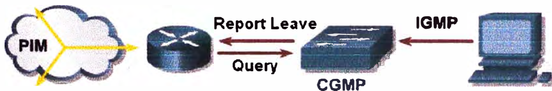
Fig. 3.9 Frame Switching CGMP Multicast Capa 2
