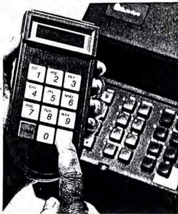
*The PIN Pad 101 security device works with the TRANZ 330™ and TRANZ 340™ systems and with all ZON II™ systems. It gives you maximum protection against debit card fraud in an easy-to-use compact package.*
