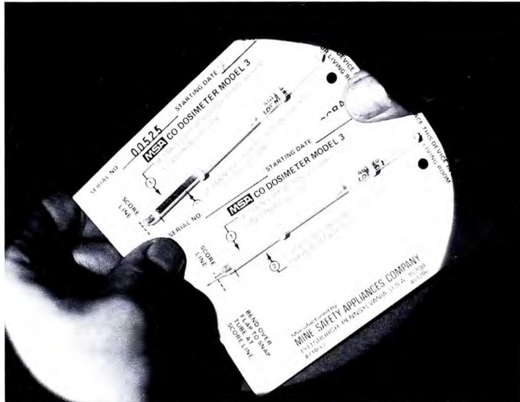
*A dark staining of the silica gel column (top Dosimeter) past one or both calibration arrows indicates a time-weighted average CO concentration exceeding 35 ppm in the ambient atmosphere.*
