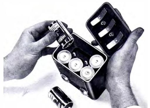
Separate battery compartment prevents exposure of components during cell replacement, protects other electrical components in event exhausted cells are left in the instrument.
