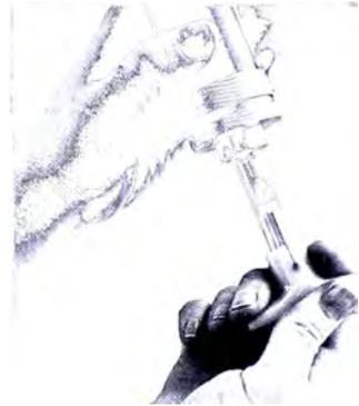
*Precision 4-position calibrated shaft accurately indexes the intake volume control at 25, 50, 75, or 100 cc; spring-loaded stop locks shaft in desired position.*
