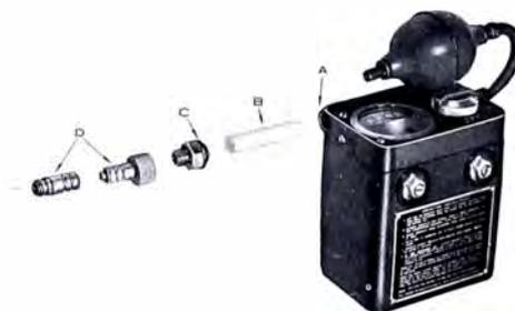
(A) Built-in filter chamber, normally fitted with (B) cotton filter to block dust, moisture; (C) sampling line connector (D) sampling line.
