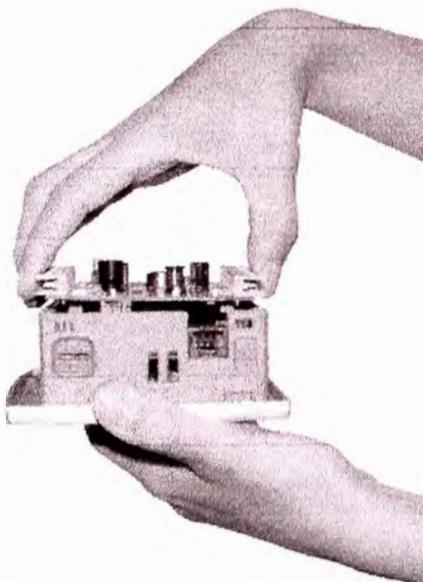
1. To access the communication jumpers, hold the I/O PCB board by its top and bottom connectors and steadily pull the board off.
