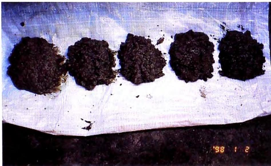
FOTOGRAFIA N°4 DE IZQ. A DER. CONCRETO PATRON, CON 10%, 15%, 20 % Y 25% DE CENIZA
