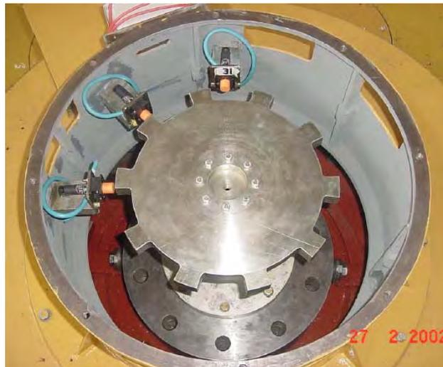
RUEDA DENTADA ACOPLADA AL EJE DEL ROTOR Y TRES SENSORES DE PROXIMIDAD
