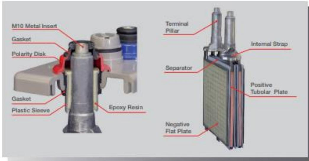
THE UNIQUE FIAMM TERMINAL DESIGN OF THE 2V CELL PERMITS PILLAR GROWTH DURING CELL LIFE WITHOUT LEAKAGE. THIS FEATURES AVOID MECHANICAL STRESS ON THE LID OF THE CELL.
