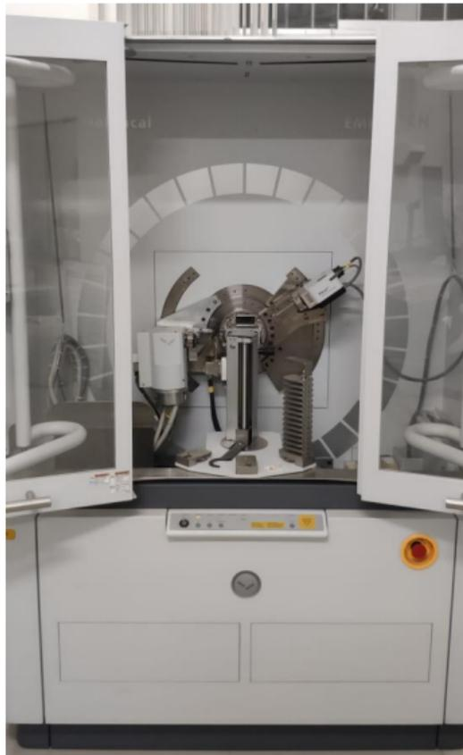
FIGURA N°3. DIFRACTÓMETRO DE RAYOS X (MALVERN-PANALYTICAL EMPYREAN ALPHA)
