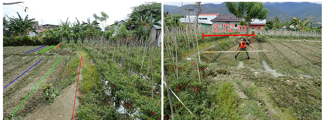
Fig. 4. Illustration of the surface rupture caused by the 2018 Sulawesi Indonesia earthquake in an agricultural field. Left: Illustration of the discontinuity in the linear arrangements of crops due to the fault rupture. Right: Measurement of the deformation across the fault line. Photos provided by Koshimura et al. (2019). The locations of the photos are shown in Fig. 5c.
