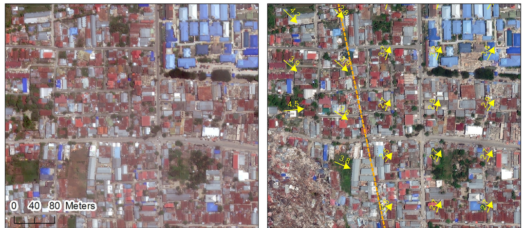
Fig. 3. Portion of the urban area of Palu city, Indonesia, captured by DigitalGlobe's sensor on July 4, 2018 (left), and October 2, 2018 (right), that is, before and after the earthquake, respectively. The orange dashed line in the right figure denotes the location of the fault line. The numbers and arrows in yellow denote the magnitude (in meters) and the orientation of the horizontal offset component, respectively. The location of the area is shown in Fig. 5c. (For interpretation of the references to color in this figure legend, the reader is referred to the web version of this article.)
