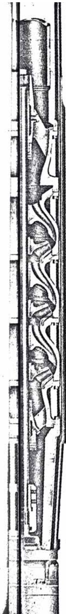
In the standard submersible turbine, bowl bearings are water lubricated. Under normal well conditions, these high quality bronze bearings last for years. But in sandy wells or where calcite build-up is a problem, bearings won't stand up.
